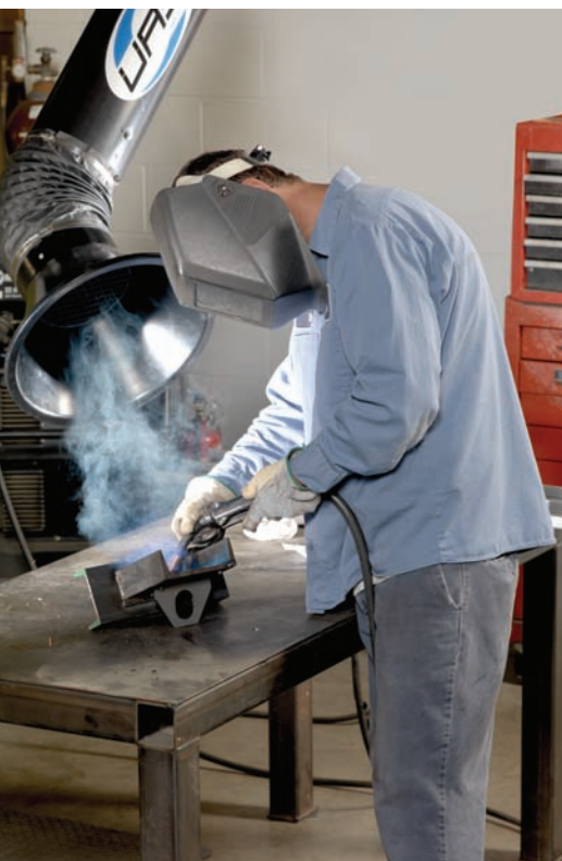
Fig. 1 — Capturing the fume at the source, as shown here, yields the best results and requires the least amount of energy.
